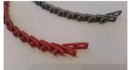
*\*All belts require adjustment, some once other a couple of times, depending on the environment they work in. Belt should be shorter then calculated length. When it comes to the power-belt, 1% is equal to 1 link per meter belt.*
